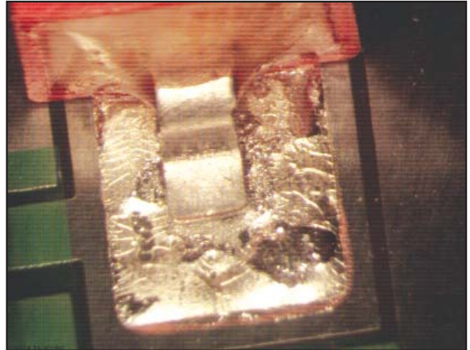
Figure 3B: Poor Wetting
