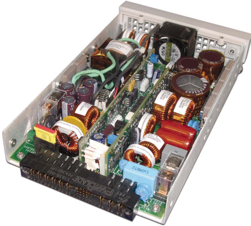
Figure 7: 500 Watt Inverter With Cooling Fan on Front Panel
