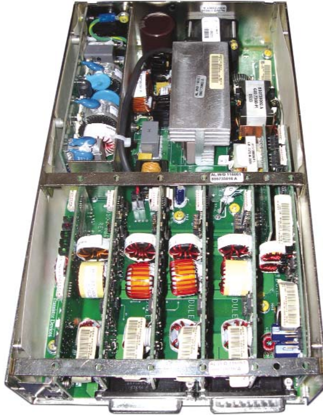
Figure 6: Multiple Output Power Supply Note the Cooling Fan on the Front Panel
